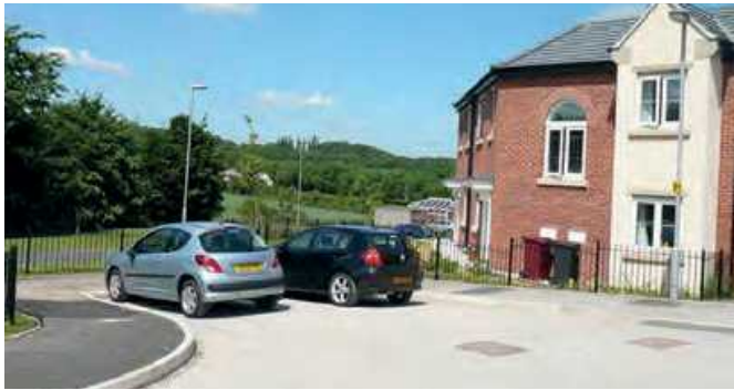
Cars parked within a turning head cause an obstruction to service vehicles needing to turn.
